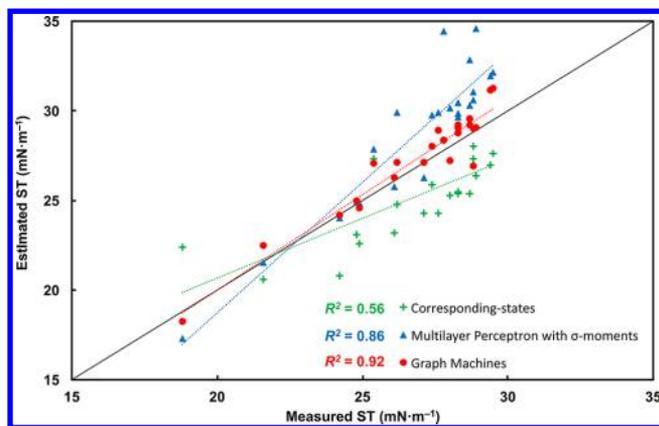
**Figure 6.** Predicted surface tension values computed by graph machine (red circles), neural networks based on five  $\sigma$ -moments (blue triangles), and corresponding-states (green crosses) vs experimentally measured surface tension values for the test set of 23 cosmetic oils.
