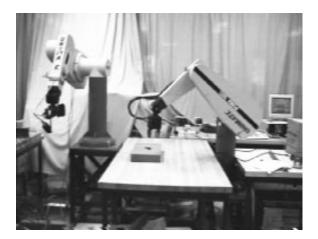
*Figure 3.* The experimental system, (a) consisting of the perceptual robot (left) and the grasping robot (right). The perceptual robot first scans the unknown object to yield a range image. A set of parameters is found which best fits the range data and this is used as a perception input to the learning system. The grasper then attempts to pick up the object based on the percept plus its acquired knowledge about the effectiveness of different grasp approach directions.
