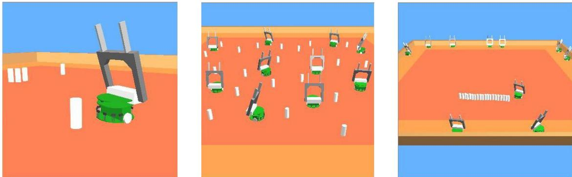
Figure 1 *Left*: close-up of a simulated robot equipped with a gripper, ready to grip a seed. *Center*: corresponding setup in the embodied simulator (10 robots, 20 seeds,  $178 \times 178 \text{ cm}^2$  arena). The inner area represents the working zone and the surrounding area is the parking/resting zone where robots that decide to stop working stay idle. *Right*: typical end of aggregation experiment, e.g., 5 hours of simulated time, in a  $178 \times 178 \text{ cm}^2$  arena.
