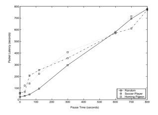
Figure 8: Mean for relay packet delivery latency on the 3 movement models for 50 nodes. evident from this distribution, the MRP is able to deliver packets at a higher delivery ratio, though it trades this capability for increased latency of packet delivery. Still, we see that over 90% of the packets are delivered in under one minute, and all are delivered in under six minutes. For many messaging applications, where eventual delivery is more important than low latency,
