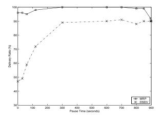
Figure 4: Packet delivery ratio v/s pause time for MRP-enhanced DSDV (MRP) and DSDV on the *Random Movement Model* for 50 nodes. intermediate node between the relay node and the destination node, therefore no opportunity for multiple relays.
