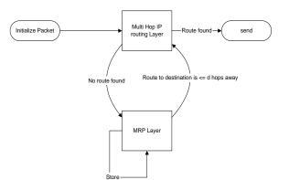
Figure 1: Integration of the MRP Protocol with a traditional ad hoc IP Routing Protocol
