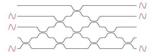
Figure 1: Schematic of a boson sampling experiment. Photons are injected (on left-hand side) into a network of beamsplitters that are set up to generate a random unitary transformation. They are detected on the right-hand side according to a probability distribution conjectured to be hard to sample from classically.
