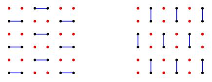
Figure 3: The architecture proposed by the quantum-AI group at Google to demonstrate quantum supremacy consists of a 2d lattice of superconducting qubits. This figure depicts two illustrative timesteps in this proposal. At each timestep, 2-qubit gates (blue) are applied across some pairs of neighbouring qubits, and random single-qubit gates (red) are applied on other qubits.
