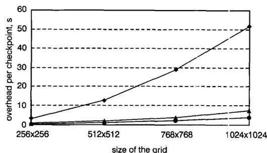
Fig.2 Overhead per checkpoint of NBC (—●—), PBC (---◆---) and DBC (---▲---) (SOR application)
