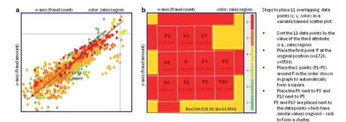
**Figure 3:** (a) Traditional scatter plot with overlapping data point P is overlapped by P–P10; (b) Variable binned scatter plot without overlapping data point P1–P10 are order and placed around P to from a red square cluster.
