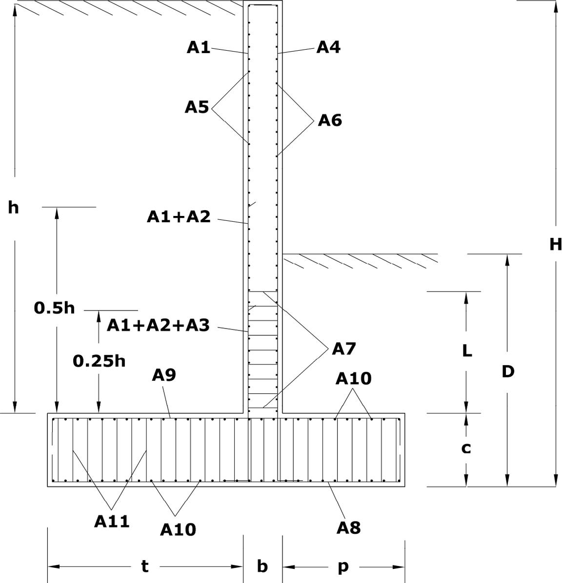
Fig. 1. Variables for the RC cantilever retaining wall
