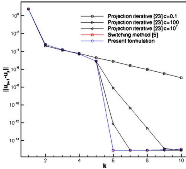
Figure 2. Iteration history of the relative difference  $\delta_k = \|u^k - u^{k-1}\|_2$ .
