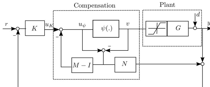
Fig. 1: Configuration for anti-windup and directionality compensation.
