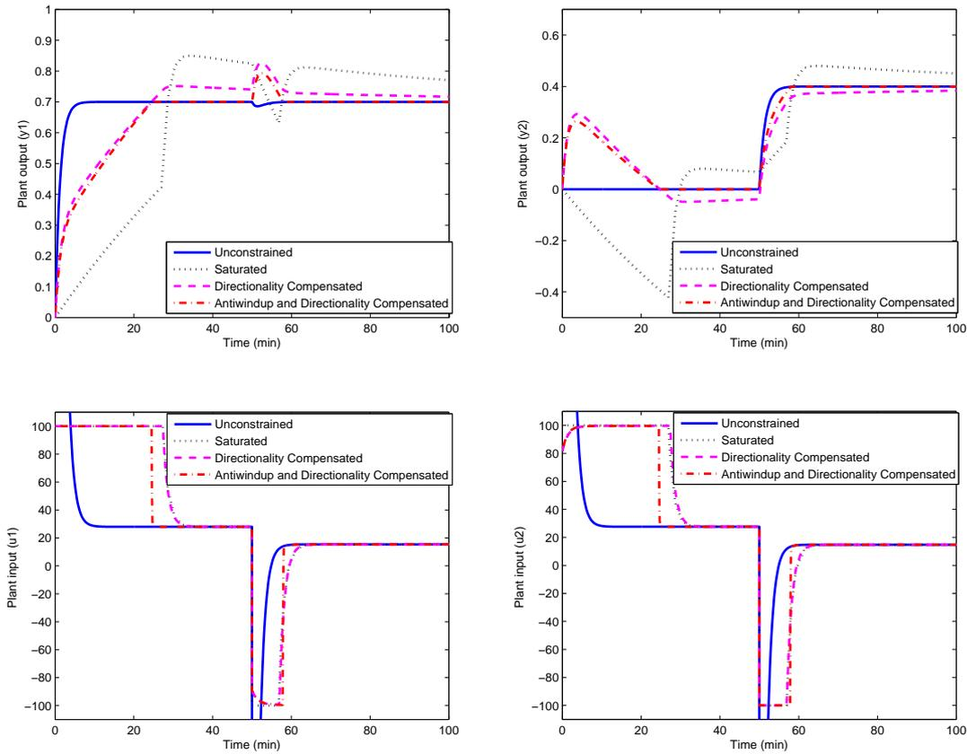
Fig. 5: Responses of the unconstrained (solid), saturated (Dotted), directionality compensated [12] (Dashed) and anti-windup with directionality compensation (Dashdotted) to a step reference. The superior performance of the anti-windup with directionality compensation over [12] can be attributed to its efficiency and swiftness in recovering linear performance after a period of nonlinear operation.
