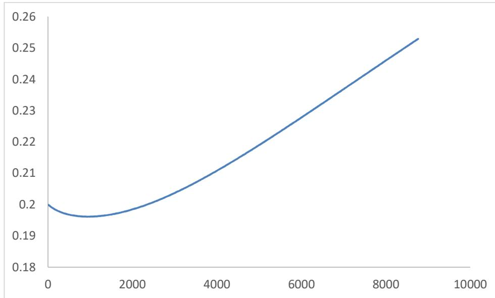
Figure 3. The expected throughput rate with time of a dehydrator when it starts from state 6.
