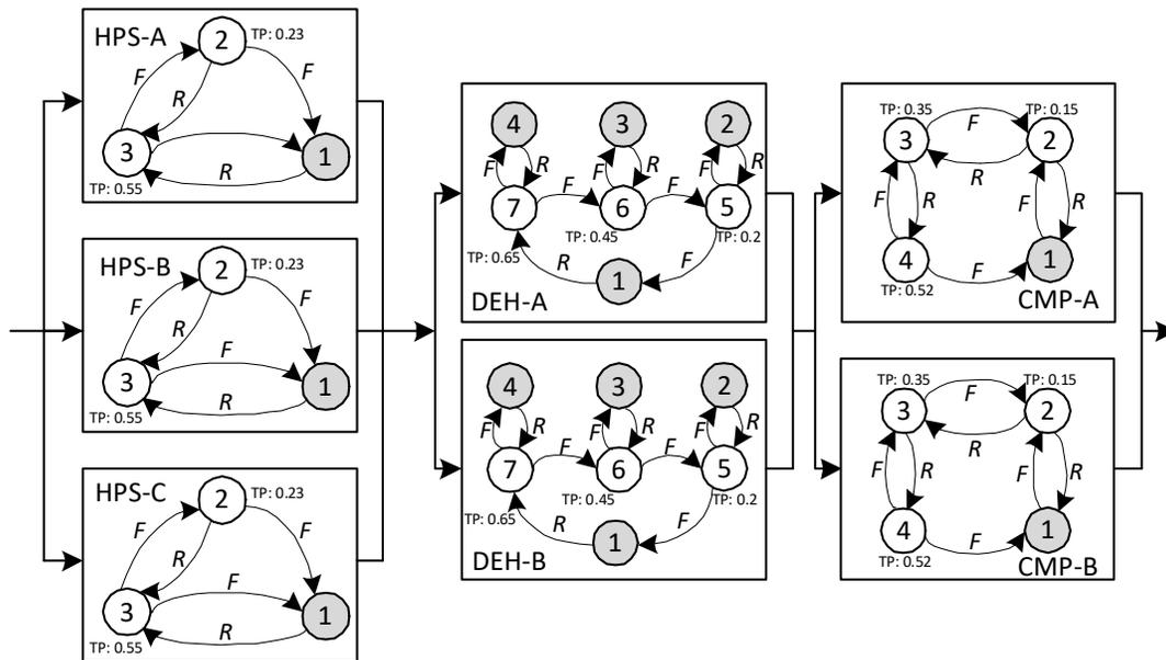
Figure 2. A Markov driven block diagram for the offshore production system
