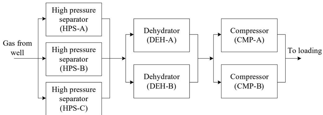
Figure 1. An offshore production/processing system
