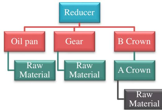
Figure 1. BOM structure for reducers and assembly.
