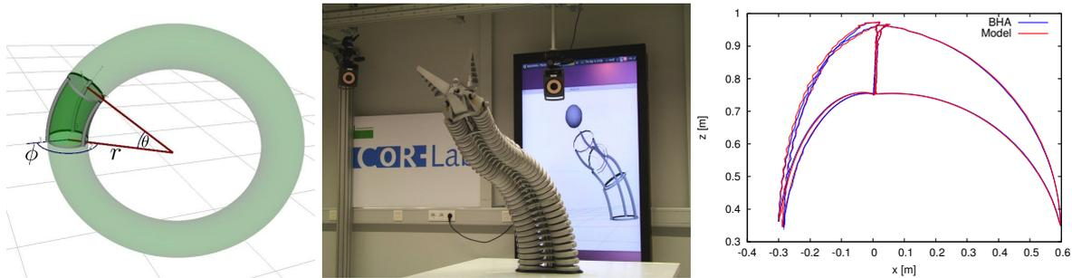
Figure 3. Kinematic simulation: Segment model including geometric parameters (left), posture example along with visualization based on the simulation model (center), and evaluation of the model quality for exemplary movements (right).
