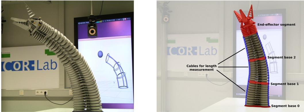
Figure 1. The bionic handling assistant BHA (left). The segments and respective length sensors of the BHA (right).
