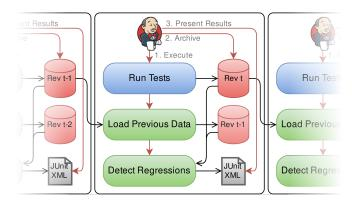
**Figure 6.** Integration of the testing framework in the Jenkins CI server. Each black rounded box represent a single Jenkins build and therefore execution of the tests for a component. Time and component versions progress from left to right.
