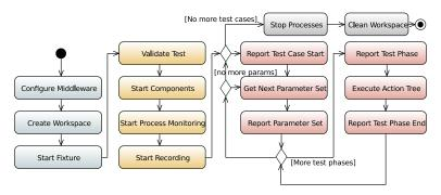
Figure 4. Visualization of steps performed to execute a performance test. Cyan: environment setup, orange: test setup, red: test case execution, gray: clean up.
