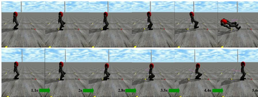
Fig. 12. COMAN robot walks through the narrow space with limited height. The top arrow demonstrates that the robot collides with the obstacle and falls down because of no usage of height variation or upper-body rotation. The below arrow demonstrates that the robot walks across the narrow crouch by reducing CoM height and rotating upper-body.
