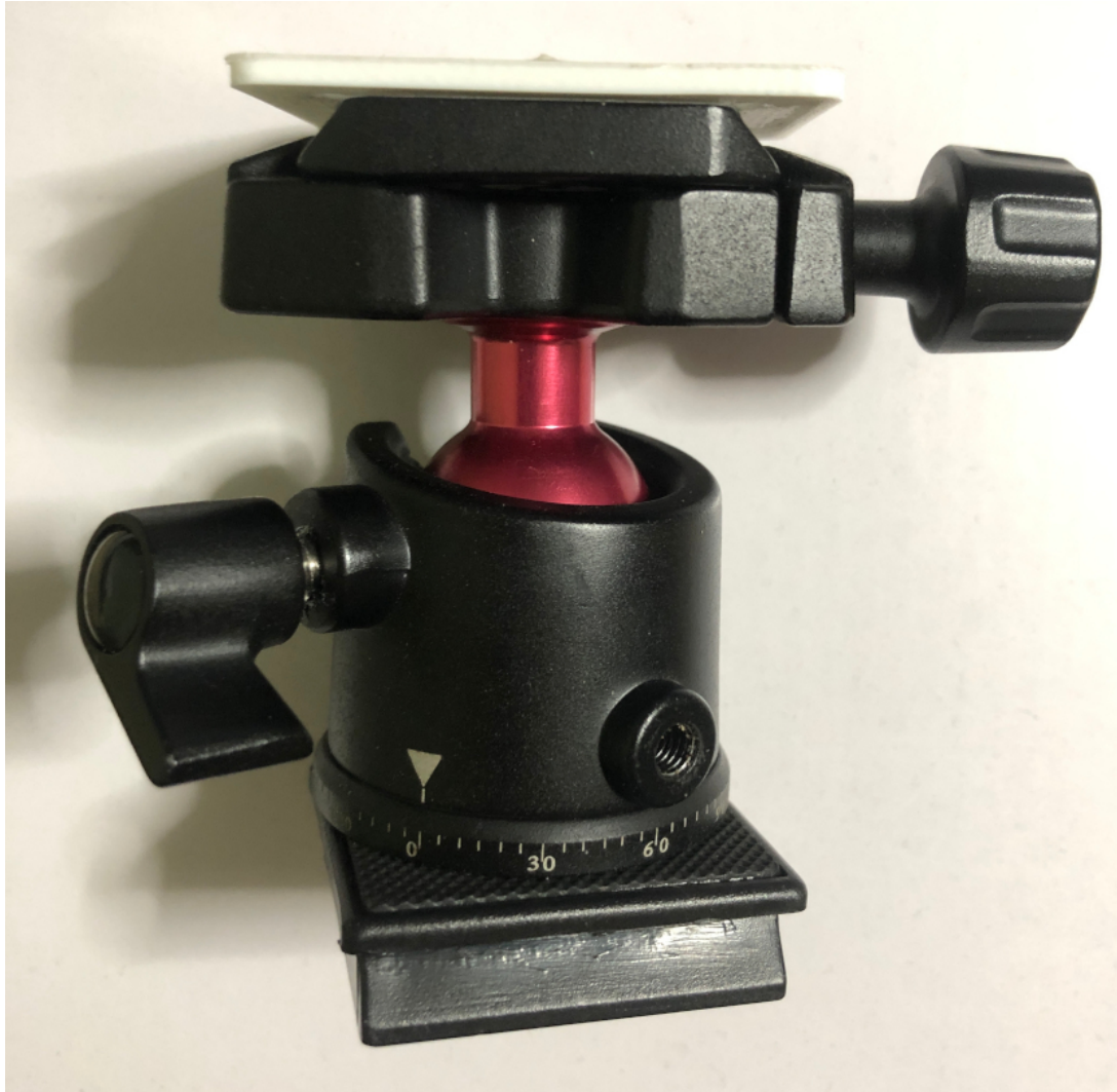
Figure 12. Angle Scale Mounted on the Tripod Used During the Experiment
