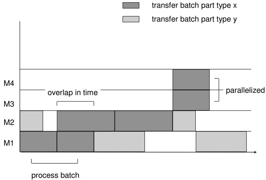
Fig. 1 Scheduling transfer batches in a modern job shop
