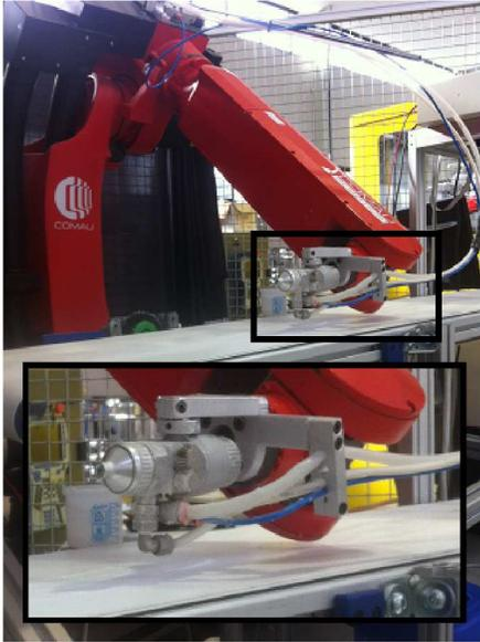
**Figure 13.** Robotic arm in a dangerous pose after following an incorrect normal.
