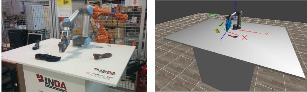
Figure 8. a) Offline adhesive spray of shoe soles. b) Shown in the simulator.
