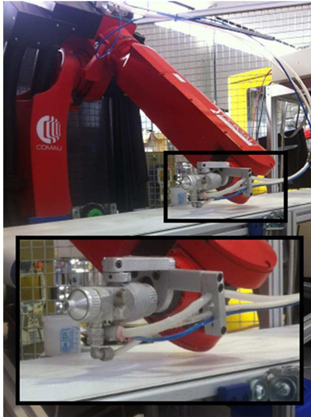
Robotic arm in a dangerous pose after following an incorrect normal.
