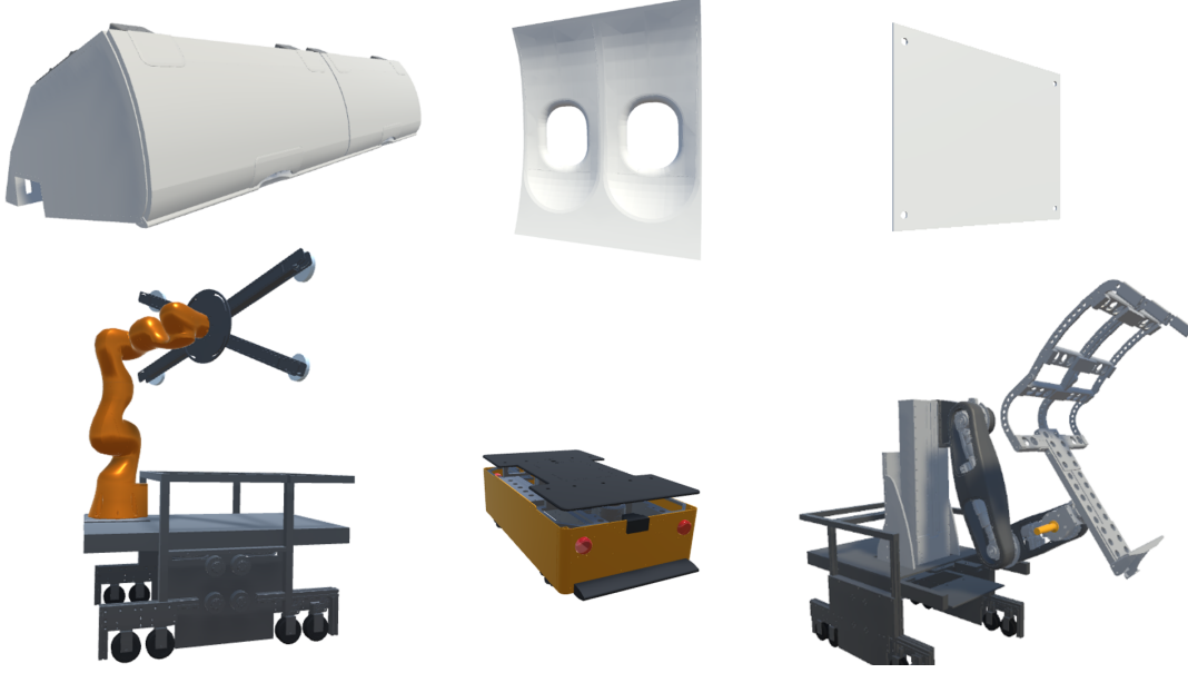
Figure 7. Assembly parts and automated systems. Top row: Hatrack, sidewall panel and lining. Bottom row: robot arm, AGV, and empowering arm.
