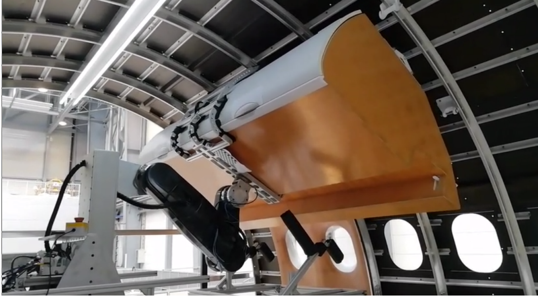
Figure 4. The heavy payload collaborative robot module while assembling an hat-rack
