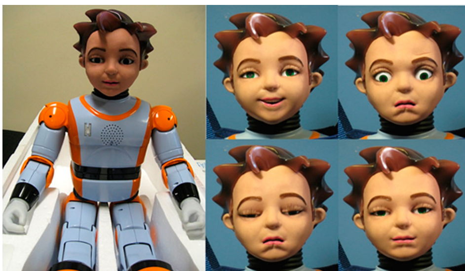
Figure 1. The Hanson Robokind Zeno R50 robot with example facial expressions.
