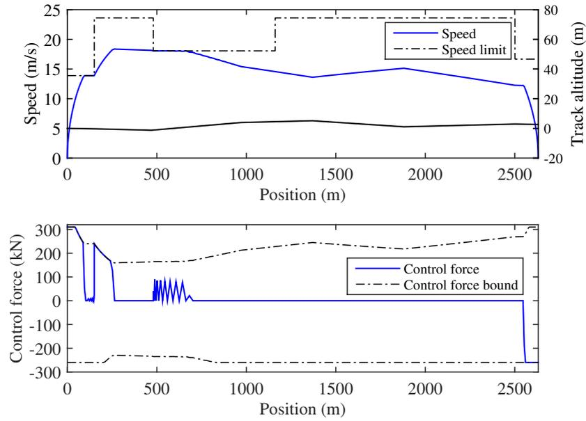
**Figure 6.** Optimal speed and control trajectories from Algorithm IV ( $T = 190$  s).
