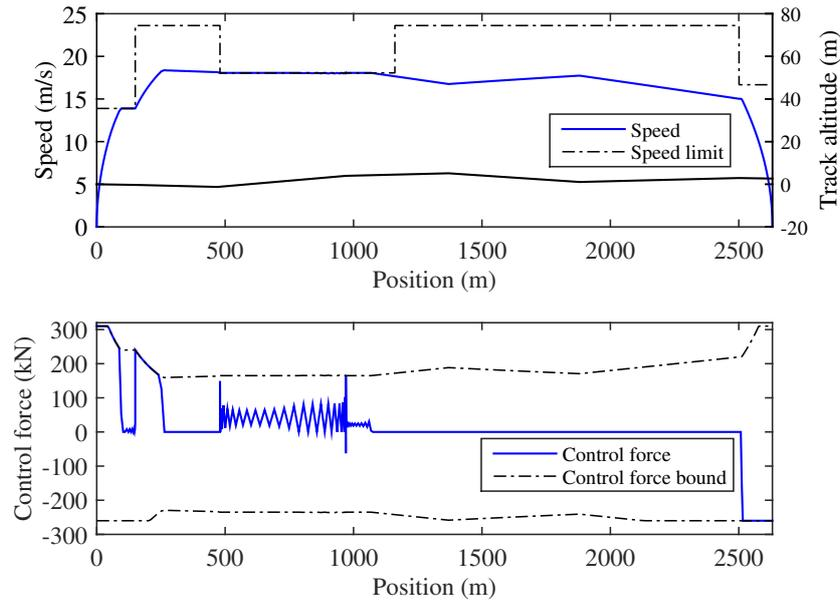
**Figure 8.** Optimal speed and control trajectories from Algorithm IV ( $T = 170$  s).
