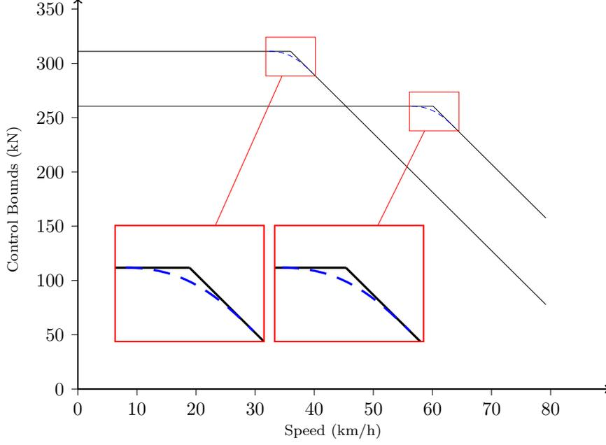
**Figure 4.** Shapes of the original (non-smooth) and approximate (smooth) control bounds for the locomotive in [18].
