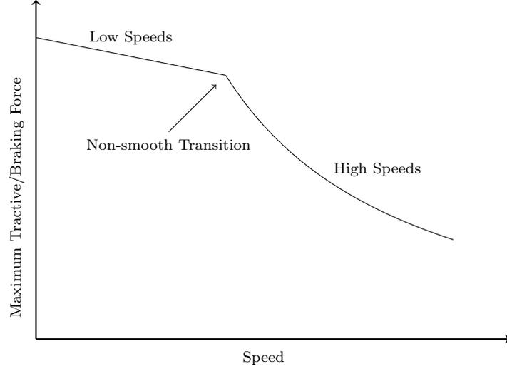
**Figure 1.** Shape of the upper bounds for the tractive and braking forces.
