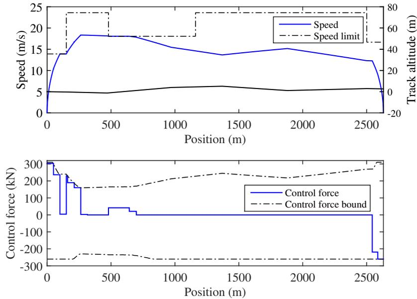
**Figure 5.** Optimal speed and control trajectories from Algorithm I ( $T = 190$  s).
