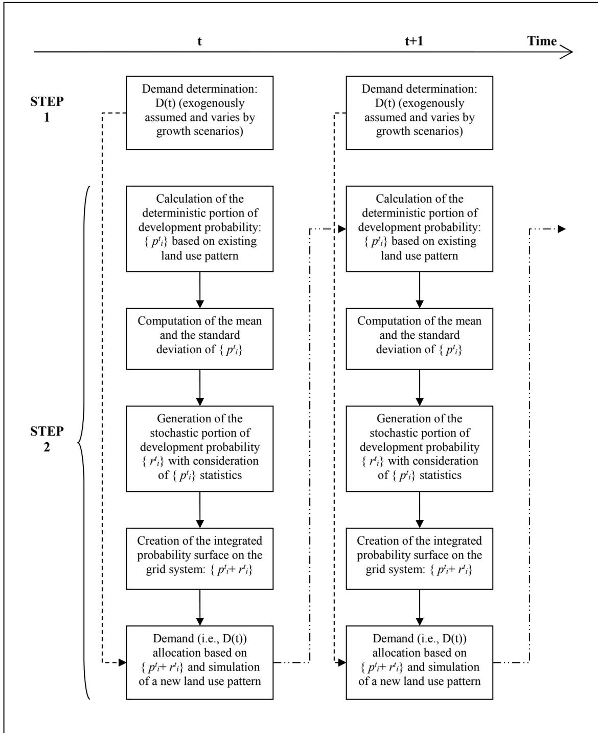
Figure 2. Experimental Simulation Procedures
