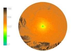
Figure 2. Example of raster map, showing the result of a path-loss calculation from an isotropic source.
