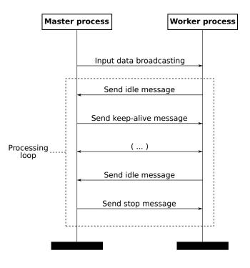
Figure 8. Communication diagram, showing message passing between master and one worker process.
