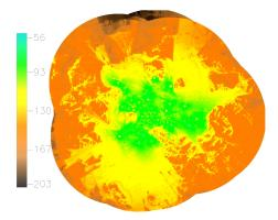
Figure 4. Example of a raster map, displaying the final coverage prediction of 136 transmitters over a geographical area. The color scale is given in dBm, indicating the received signal strength. Darker colors denote areas with a reduced signal due to the fading effect of the hilly terrain and clutter.
