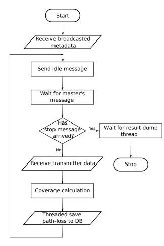
Figure 7. Flow diagram of a worker process.
