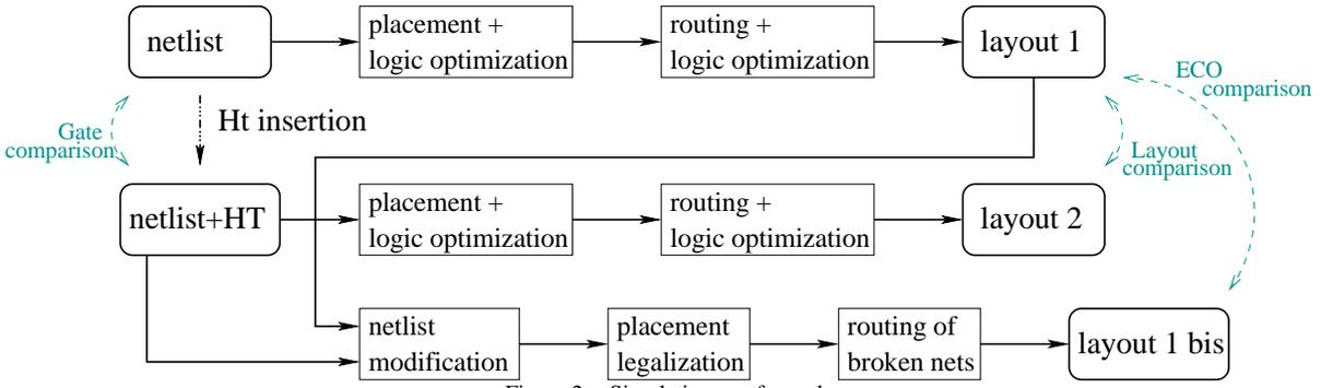
Figure 2. Simulations performed
