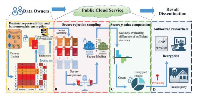
Fig. 2. The workflow of the proposed HEALER framework involving four key steps: Step A: Data preparation and encryption by data owners, Step B: Secure rejection sampling in public cloud, Step C: Secure-value computation in public cloud, and Step D: Result dissemination to authorized researchers (Color version of this figure is available at *Bioinformatics* online.)
