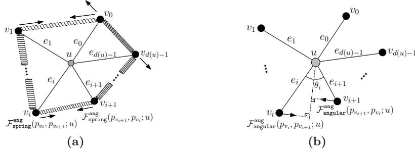
**Fig. 3:** Forces applied on nodes in order to maximize the angular resolution. (a) Springs on consecutive edges around  $u$ . (b) Repelling or attractive forces based on the angles.
