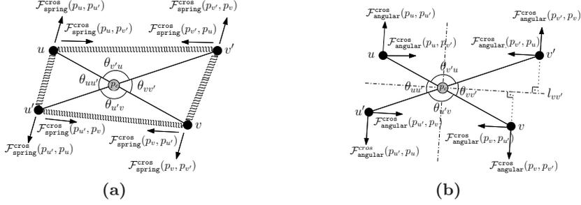
**Fig. 2:** Forces applied on nodes in order to maximize the crossing resolution. (a) Springs on nodes involved in crossing. (b) Repelling or attractive forces based on the angles.
