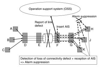
Fig. 8 Alarm suppression by AIS.
