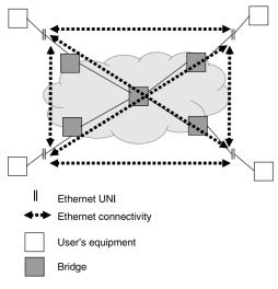
Fig. 2 Example of multipoint-to-multipoint TLS.
