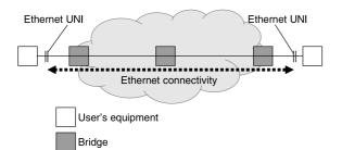
Fig.1 Example of point-to-point TLS.
