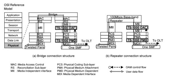
Fig. 2 Typical TS-1000 protocol stack structure.
