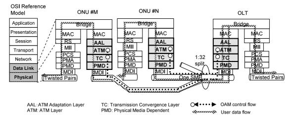
Fig. 3 B-PON deployed in Japan protocol stack structure.
