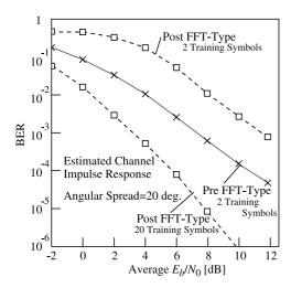
Fig. 7 BER of post-FFT and pre-FFT type array antennas.
