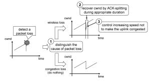
Fig. 3 Overview of the proposed mechanism.
