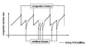
Fig. 4 Expected changes in congestion window size with our mechanism.
