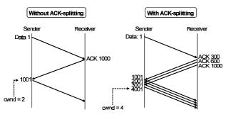
Fig. 2 Time chart of ACK-splitting during slow start phase.
