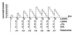
Fig.5 Typical changes in the number of ACK packets for each data packet.
