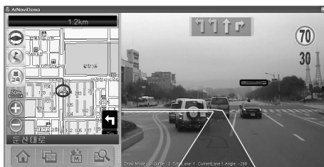
Fig. 9 Snapshot of the video-based car navigation system (CNS) which includes the proposed traffic light detection module. The blue box in the center represents the detected traffic lights.
