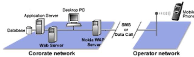
The Operator network accesses the WWW and corporate servers to optimise the data that will be transmitted through the wireless (operator) network. WAP can operate on all wireless networks available. The corporate network (or an Internet ISP) links to the operator's network (and therefore the mobile device) through a data call. The network will need access to a WAP server for the conversion of the data, as shown in the corporate network above.
