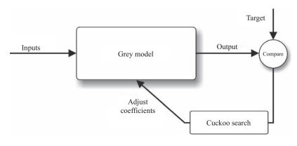
Figure 1. Schematic diagram of CS-based Grey model
