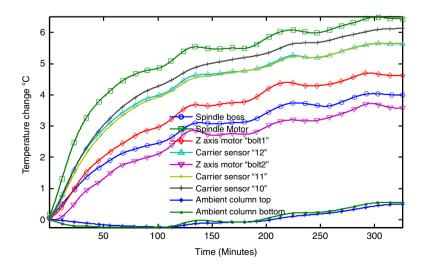
Figure 3. Measured temperature variation (model inputs)
