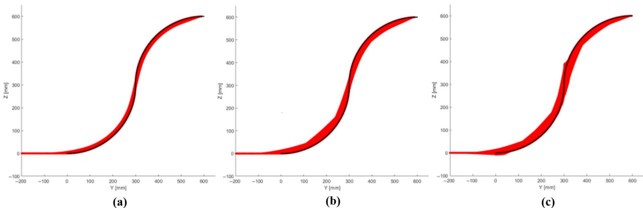
**Notes:** (a) Envelop of path-following method without joint limits; (b) envelope of pathfollowing method with joint limits; (c) envelope of numerical method
