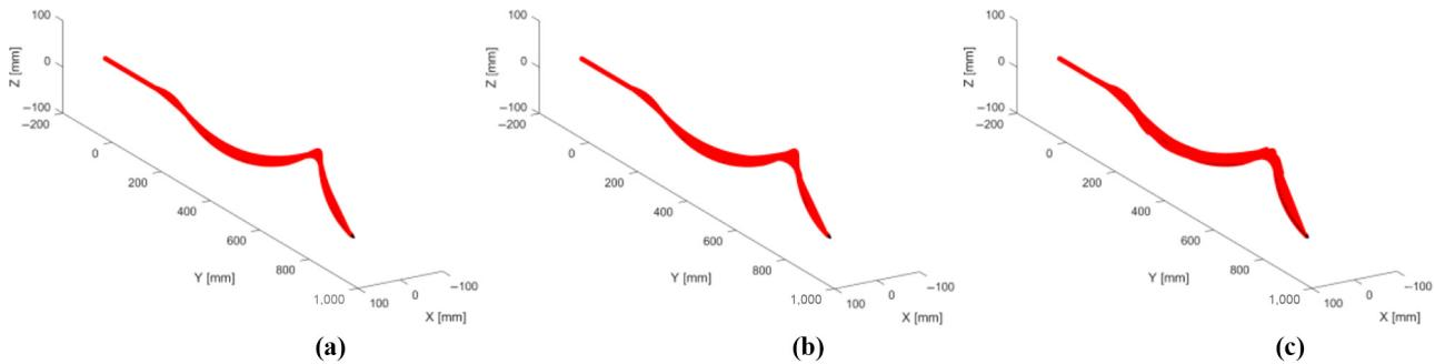
**Notes:** (a) Envelop of path-following method without joint limits; (b) envelope of pathfollowing method with joint limits; (c) envelope of numerical method
