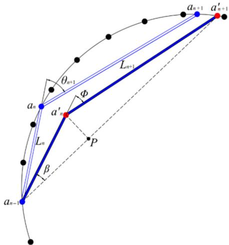
Thus, the position of  $a'_{n+1}$  can be calculated by the same method in Section 3.2 or 3.3 with the chord length of  $|a_{n-1}a'_{n+1}|$ . According to space analytic geometry, the position of point  $P$  can be obtained as [equations \(14\) \(15\) \(16\)](#):
