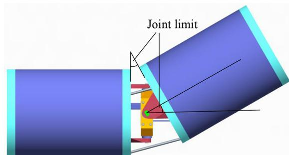
**Figure 7** Incorporating joint constraints within path-following method
