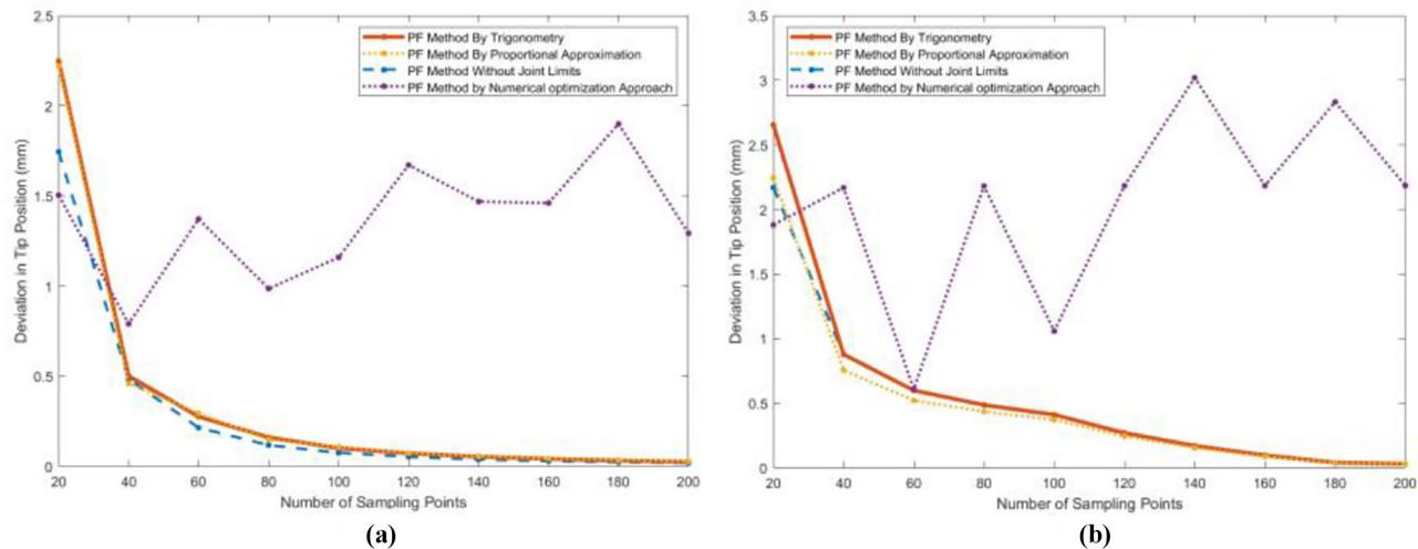
**Notes:** (a) Maximum deviation of pathfollowing methods for S-bends path; (b) maximum deviation of path-following methods for helix path
