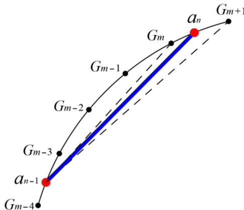
**Figure 4** Illustration of finding joint points by trigonometry
