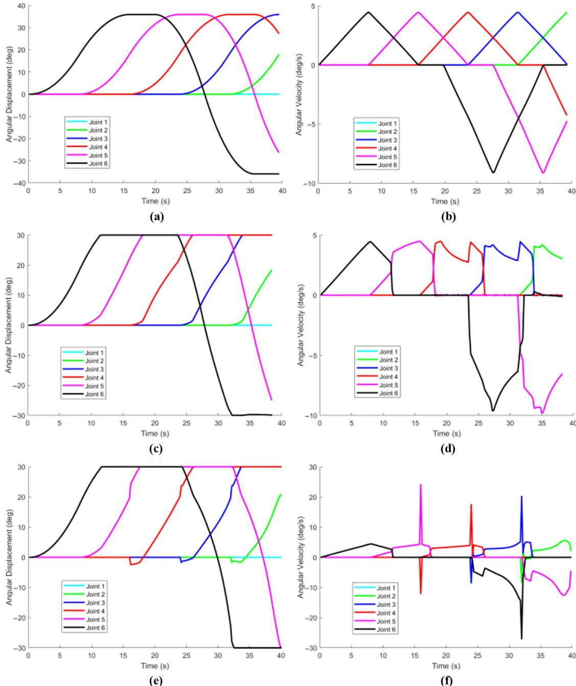
**Notes:** (a) Angular displacement of path-following method without joint limits; (b) angular velocity of path-following method without joint limits; (c) angular displacement of path-following method with joint limits; (d) angular velocity of path-following method with joint limits; (e) angular displacement of numerical path-following method; (f) angular velocity of numerical path-following method
