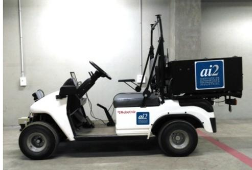
Figure 2. Car-Like mobile robot
