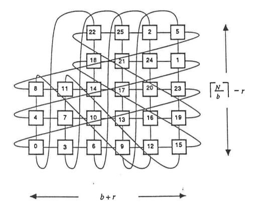
Figure 4. Midimew network with N = 26 and b = 4 (r = 2).
