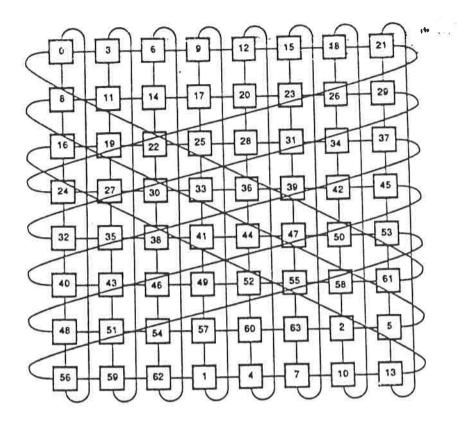
Figure 7. Square mesh for N = 64 with hops 3 and 8.
