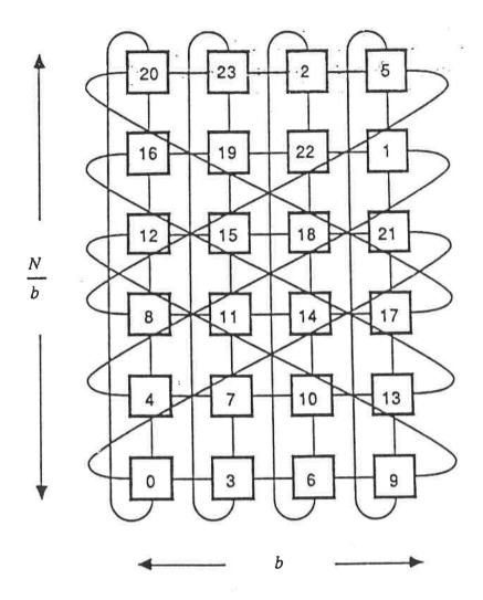
Figure 3. Midimew network with N = 24 and b = 4 (r = 0).
