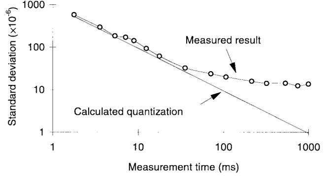
Fig. 3. Measured standard deviation versus the total measurement time.
