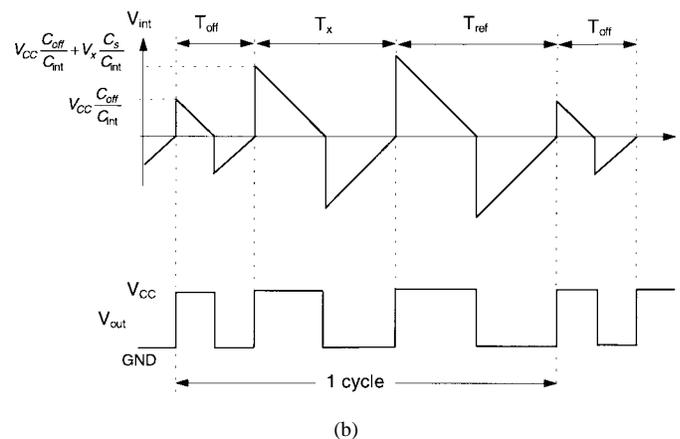
Fig. 1. (a) The schematic diagram of the interface and (b) output signals  $V_{int}$  and  $V_{out}$  of the interface.
