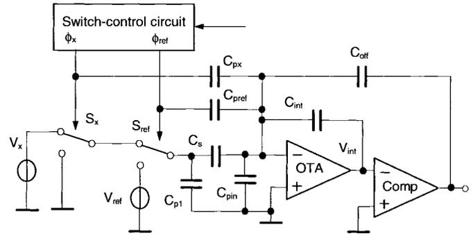
Fig. 2. The parasitic capacitances of the interface.
