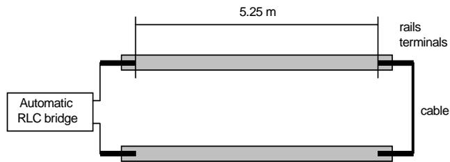
Figure 1: Measuring circuit for low current tests
