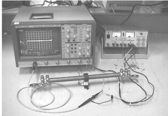
Figure 7: Hall effect sensor HFA1C300 (on the copper bar); power supply; digital oscilloscope LeCroy 9314M
