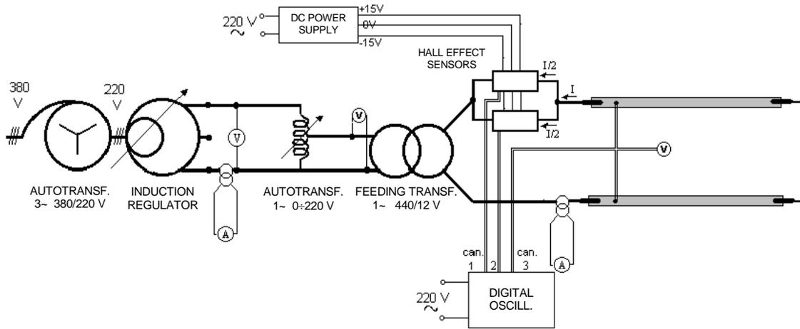
Figure 8: Measuring system for high current tests
