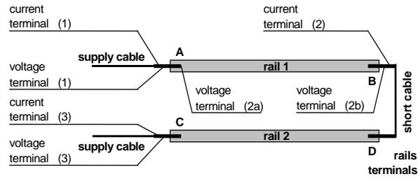
Figure 3: Configurations of voltamperometric measurements of the dc resistance of contacts and rails
