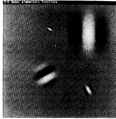
Fig. 6. Five examples of 2-D Gabor elementary functions displayed as luminance primitives. These biologically modeled "wavelets" can all be generated from a single complex member by dilations, rotations, and translations, as specified by (22).
