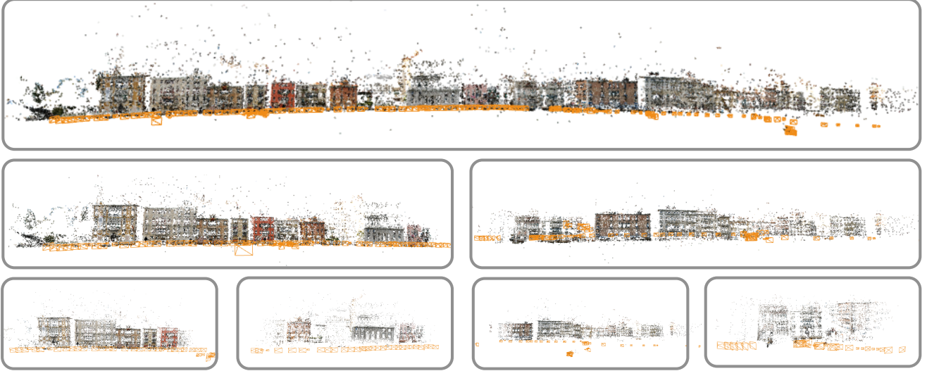
Fig. 1. We introduce HyperSfM, a divide-and-conquer approach for Structure from Motion. We represent an SfM problem by a hypergraph which we recursively partition, obtaining a tree of fully-constrained, nonlinear sub-problems. The top three levels are shown above for the "Grand Canal" data-set [1]. After partitioning, computation proceeds from the bottom up, recursively merging submaps.
