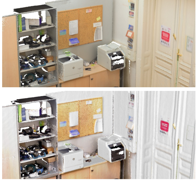
Figure 1. Top: an office scene reconstructed in HDR with the proposed exposure time controller. Note the difference in color between the wooden panel on the left, the gray wall, and the milky white door on the right. Bottom: the same scene reconstructed in LDR with ElasticFusion using a fixed exposure time setting. The dynamic range of the scene exceeds that of an LDR image; as a result the panel, wall, and door were overexposed and appear to have the same color in the reconstruction.
