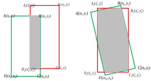
Figure 2. IoU computation for 2D: axis-aligned and rotated bounding boxes, where the green and red represent the ground truth and predicted bounding box respectively. The intersection area is highlighted in gray.
