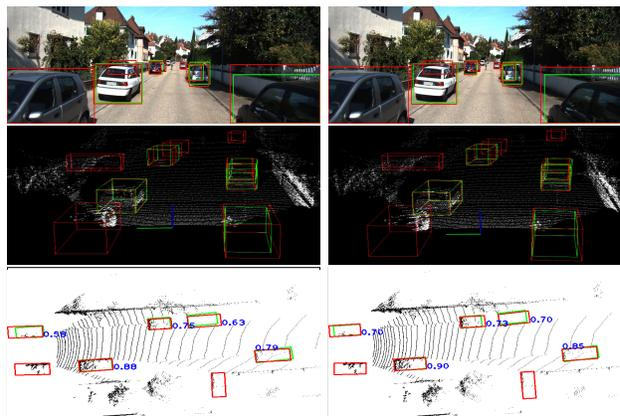
Figure 1. An example of 3D car detection results from different models trained with SECOND [10] and SECOND + proposed  $L_{IoU}$  loss are shown in the left and right columns. The IoU value for each Bbox has been provided in the Bird-eye-view image at the bottom this figure. From this figure, we can find that the accuracy of the bounding boxes has been steadily improved by using the proposed IoU loss.
