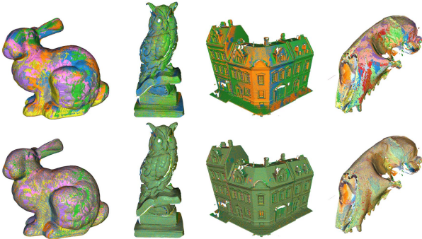
Figure 3: Color coded triangulation of the sub-scans aligned with rigid ICP (top row), and non-rigid ICP with Graph-Laplacian (GLP) based displacements (bottom row).
