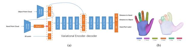
Figure 2: (a) Illustration of the generative grasping field network conditioned on an object point cloud. The red dashed arrow denotes sampling from a distribution. Network details are in Appendix A. (b) Illustration of hand part labels. Left is our hand part annotation on the MANO model. Right is an example of our *predicted* surface points with hand part labels.
