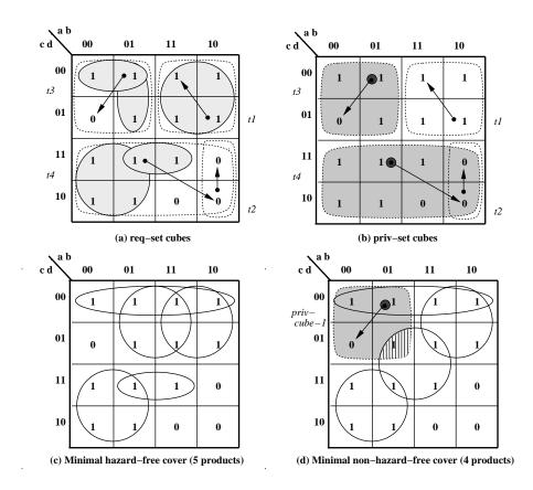
Figure 1: Two-Level Hazard-Free Minimization Example: (a) shows the set of required cubes (shaded); (b) shows the set of privileged cubes (shaded); (c) shows a minimal hazard-free cover; (d) shows a minimum-cost cover that is not hazard-free, since it contains a logic hazard.
