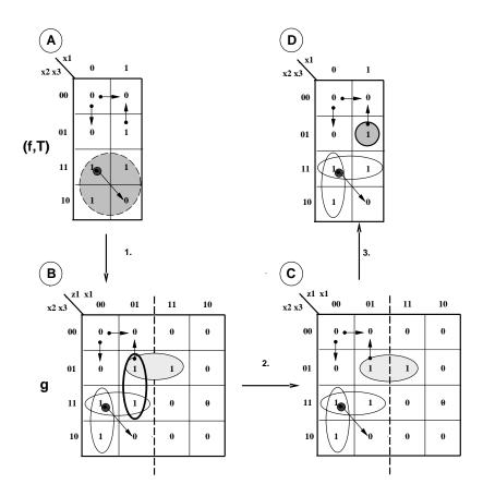
Figure 8: Example for recasting prime generation. A) shows the function (f, T) whose dhf-primes are to be computed. B) shows the auxiliary synchronous function g and its primes. C) shows primes of g that do not intersect illegally. D) shows the final dhf-primes of f, after deleting the  $z_1$  variable.
