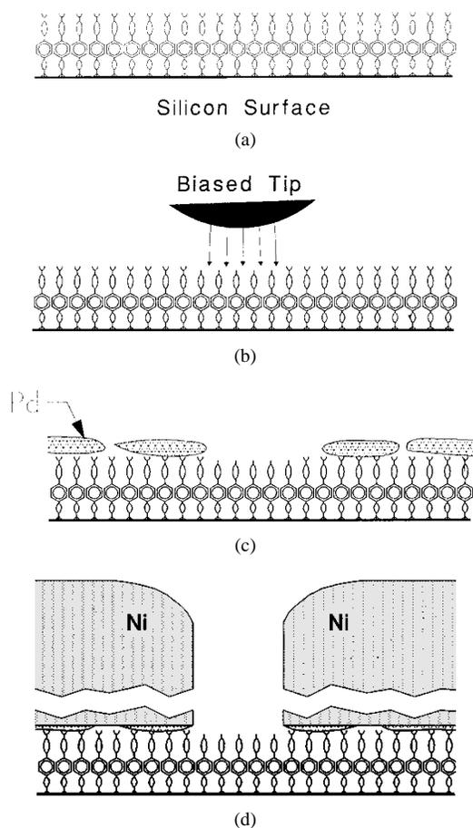
**Fig. 10.** Schematic illustrating replication of a high-resolution pattern in an STM exposed SAM film. (a) Starting SAM film, (b) pattern generation by using an STM as a source of low-energy electrons to interact with and expose the film, (c) ligation of Pd catalyst, and (d) electroless growth of Ni from solution.
