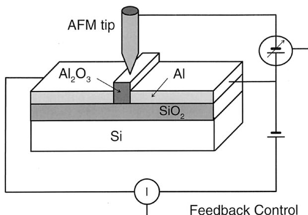
**Fig. 6.** Diagram of the circuit used for fabricating the metal–oxide device structures. The device current was measured in real time during the fabrication to guide the anodization.
