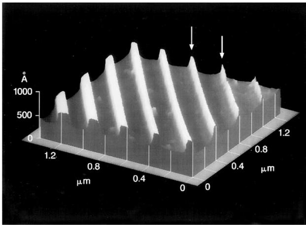
**Fig. 4.** AFM image of a pattern etched into an Si sample by using an  $\text{Cl}_2$  plasma generated by an ECR source. The etch depth was 30 nm. The two lines indicated by the arrows have linewidths of 20 and 10 nm.
