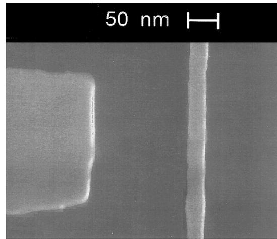
**Fig. 5.** SEM image of the active region of a side-gated transistor fabricated from SIMOX. The width of the source-drain channel is 30 nm.
