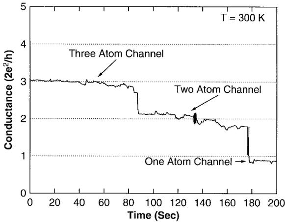
**Fig. 8.** Conductance of an  $\text{Al}/\text{Al}_2\text{O}_3$  junction as the last remaining conduction channels are cut off. The conductance is quantized in approximate units of  $2e^2/h$ . A conductance of  $2e^2/h$  corresponds to a one-atom conduction channel.
