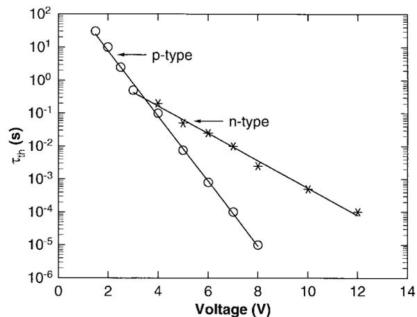
Fig. 3. Plot of the threshold exposure time  $\tau_{th}$  versus voltage for an n- and p-type sample.
