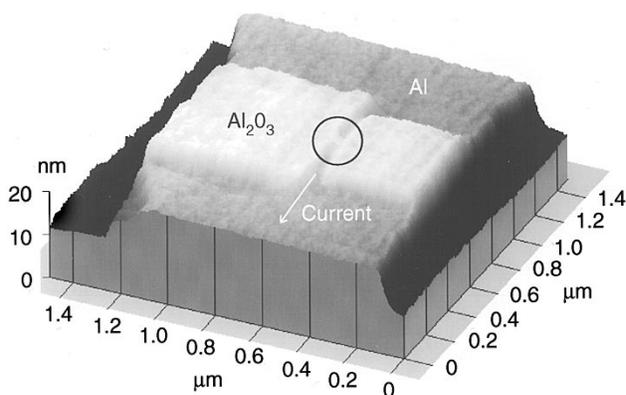
**Fig. 7.** AFM image of an  $\text{Al}/\text{Al}_2\text{O}_3$  lateral metal–oxide–metal junction. The current is first constricted down to a 40 nm-wide wire and passes through the lateral metal/oxide junction indicated by the circle.
