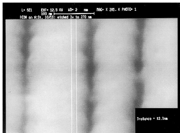
**Fig. 11.** SEM image of narrow trenches etched into Si created by the process illustrated in Fig. 10. The parallel white lines are spaced by 12.3 nm.
