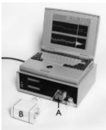
Fig. 4. Prototype FABS instrumentation. The FABS flow cell containing the cantilevers is mounted on the front (A). The electronics box contains a preamplifier, a lock-in amplifier, and a current source. The instrument also includes a small pump (B) and a laptop computer.
