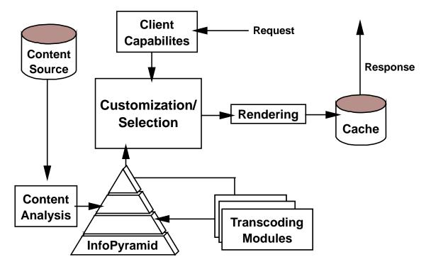
Figure 1. Internet content adaptation system architecture
