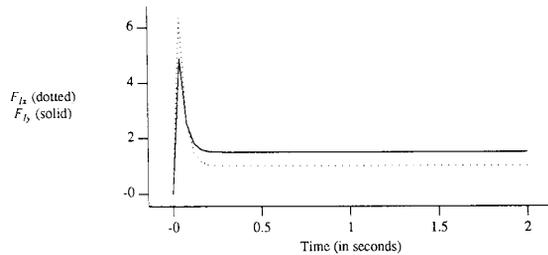
Fig. 15. Interaction forces for the circular trajectory. The desired values of  $F_{Ix}$  and  $F_{Iy}$  are 1.0 and 1.5 respectively.
