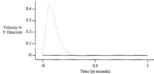
Fig. 6. Velocity in  $y$  direction for the straight line trajectory (solid line—desired trajectory, dotted line—actual trajectory).
