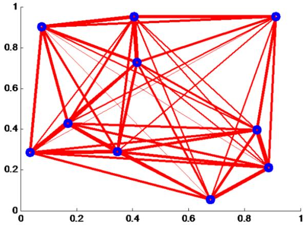
Fig. 4. Random geometric graph with 10 nodes. The width of each edge is proportional to its weight.
